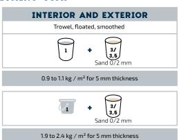
FINISHED THICKNESS approx. 5 mm: as the strengths of these render are low, scraped, raised or brushed finishes may present a risk of permanent powdering.
